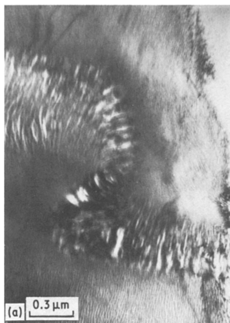
Figure 9 (a) Transmission electron micrograph of Ni 37-12 aged for 0.5 h at 873 K showing an "S" shaped secondary discontinuous reaction front. (b) Optical micrograph of Ni 48-9 aged for 200 h at 873 K showing "S" shaped secondary discontinuous reaction fronts.
